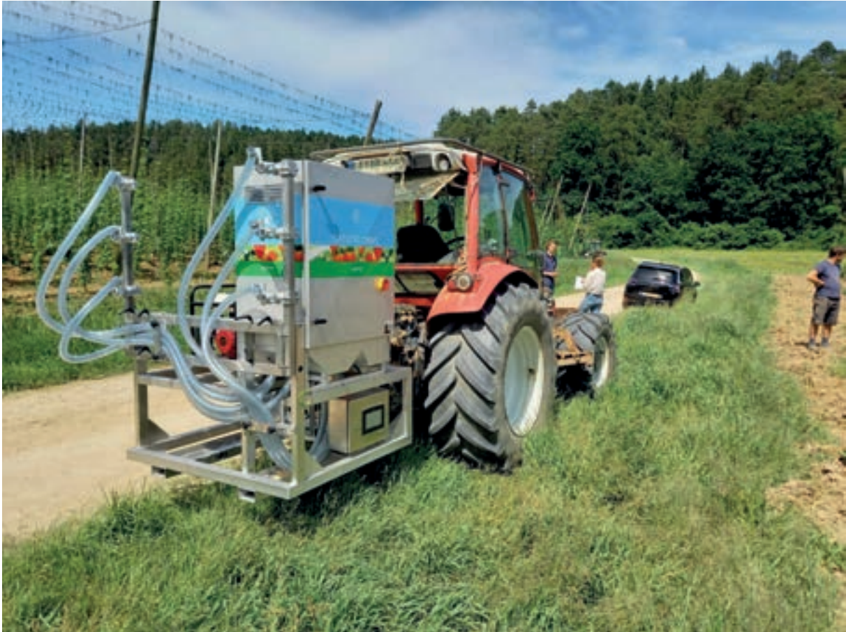
Figure 1. First Koppert prototype for the release of predatory mites in a hop garden. Dürnwind, Hallertau, Germany; Photo: FW (15 June 2021)
